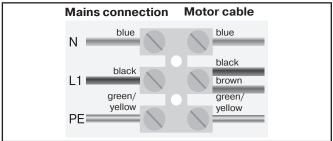
The brown wire and black wire are connected together at "L".
