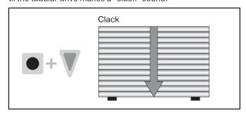
Travel to the desired upper end limit position. Subsequently press the learn button and the UP button until the tubular drive makes a "clack" sound.
