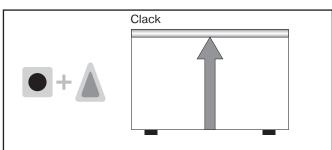
With permanent stoppers (stopper for the upper end limit or anti-lifting devices for the lower end limit), the tubular drive automatically stops during installation travel and automatically saves the end limit(s).
